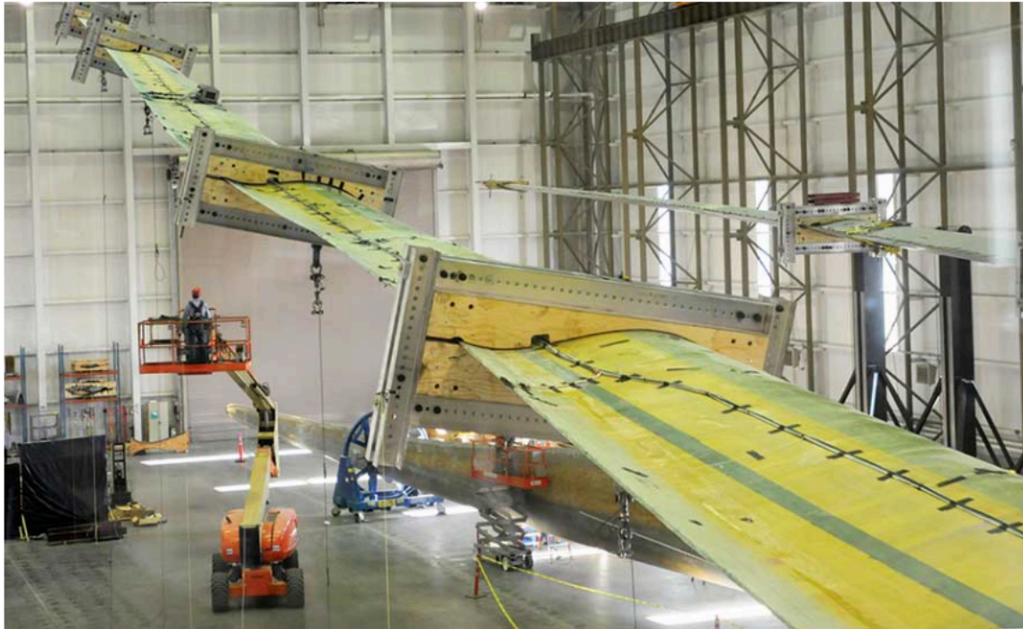
Massachusetts facility does R&D and tests turbine blades up to 90 m long to meet global design standards.
